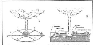
A tile system protects a tree from a raised grade. A, The tile is laid out on the original grade, leading from a dry well around the tree trunk. B, The tile system is covered with small stones to allow air to circulate over the root area.
