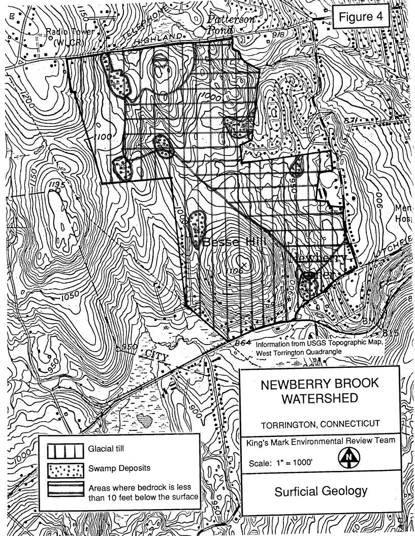
feet of the deposit and in shallow to bedrock areas. However, where till exceeds 6-8 feet in depth, a compact (siltier) layer, called hardpan, may underlie the friable till. Based on the <u>Soil Survey of Litchfield County</u>, <u>Connecticut</u>, the compact till occurs mainly in the Besse Hill area.
