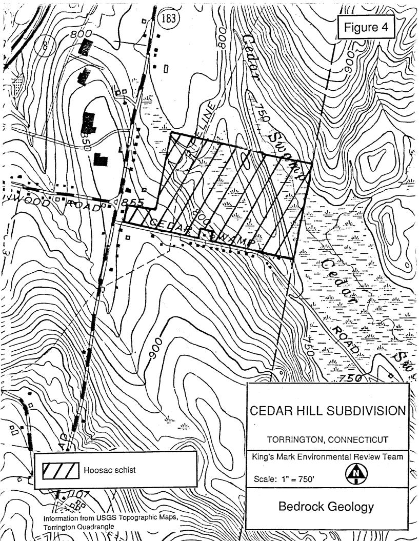
places on the site. The underlying bedrock should not pose any major problems for the proposed subdivision, unless it is encountered during excavation for roads, foundations, utility lines, etc. If bedrock is encountered, blasting may be required or large, earth moving equipment may be utilized. Based on soil and geologic mapping data and the proposed roadway layout, blasting will probably not be necessary.
