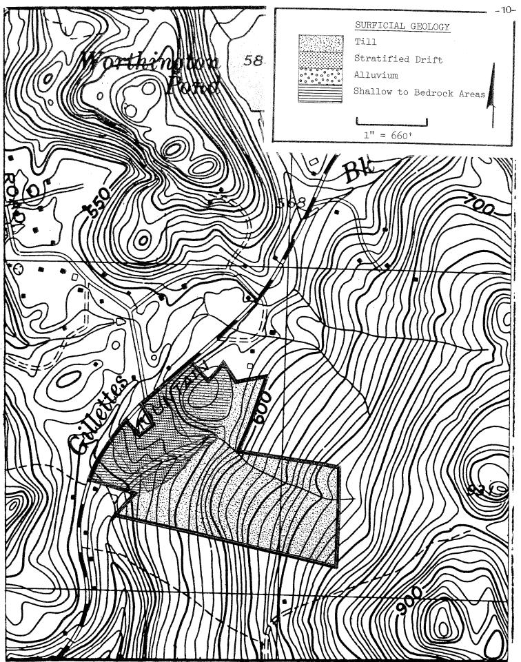
time of year. Percolation tests conducted on the site indicate the relatively slow permeability of these soil zones. Most percolation rates ranged in the area of 11 to 20 minutes per inch.
