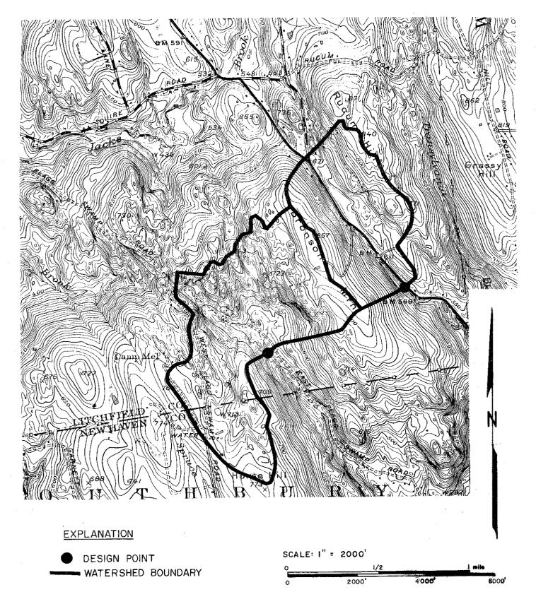
Development as proposed would generate additional runoff from the site, causing an increase in peak flows in the brooks. These increases, however, should be relatively small. Figure 4 shows the two points along the brooks at which runoff from the site may be expected to have its maximum effect on flow rates. The overall drainage areas for the brooks at those points is also shown.
