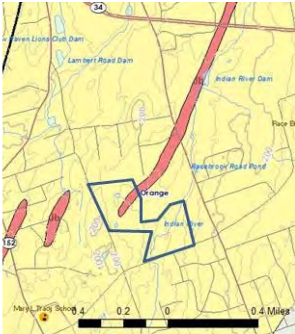
Figure 2. Geologic map (Rodgers, 1985) of the Ewen Farm Preserve and surrounding area. Area shown in yellow is underlain by Wepawaug Schist; area in red is underlain by basalt. Outcrops are not shown on this map. Outline of Preserve (blue line) very approximate.
