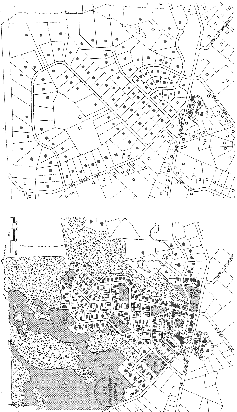
Figure 5-1. Site plan for the proposed expansion of Romansville, an historic hamlet within the rural/suburban township of West Bradford, Chester County, Pennsylvania. The author's design (at right) retains the entire density of the developer's original "cookie-cutter" plan (shown on the left) but arranges the development in a more compact village-like manner that preserves a substantial greenbelt of woodlands and farm fields around its perimeter. Due to their very compact nature, neo-traditional village layouts do not have the same high proportion of "view lots" that are commonly found in well-designed "conservation subdivisions." To compensate for this, the Romansville design includes five internal greens or commons (plus two ballfields), a relatively high number for a development of approximately 150 houselots.
