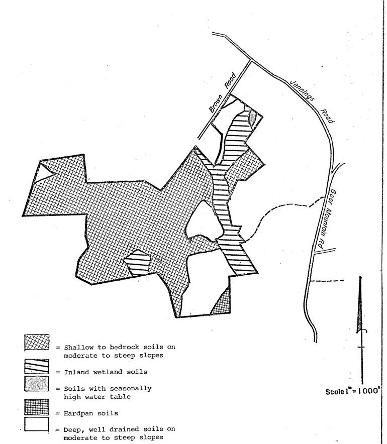
Approximately 50% of the eastern half of the site consists of deep, well drained Charlton soils according to the Litchfield County Soil Survey. These are the most suitable soils for residential development on the property. The remaining soils in the eastern half of the site consist of a mixture of hardpan soils, seasonally wet soils, wetland soils and shallow to bedrock soils (see Figure 5).
