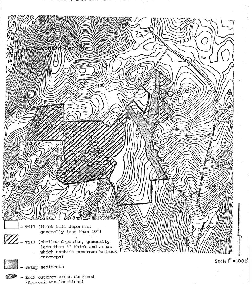
In some areas on the site, till and/or bedrock is overlain by swamp sediment. Swamp sediments consist of peat and muck interbedded with sand, silt and clay. Wetland areas on the site are designated by the symbols Le, Lc, Lg and Pm on the accompanying soils map (see Appendix).
