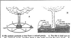
A tile system protects a tree from a raised grade. A, The tile is laid out on the original grade, leading from a dry well around the tree trunk. B, The tile system is covered with small stones to allow air to circulate over the root area.
