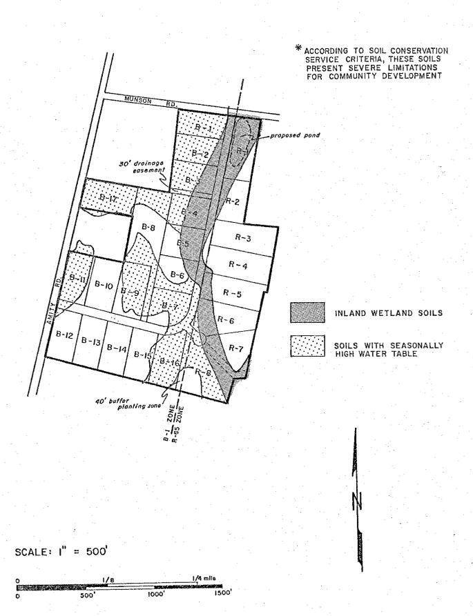
Due to the problematic soils of much of this site, it is recommended that a complete erosion and sediment control plan be prepared for this site. This should show typical design sections; standards and specifications for measures to be installed; seeding recommendations including varieties of seed, seeding rates and time of seeding; and lime and fertilizer recommendations including fertilizer analysis and rates of application.
